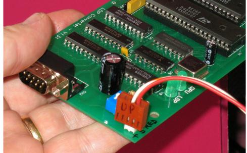
\*\*\* +5Volts is supplied to the LaserCon board through this connector. Make certain that the red wire is on the correct side which is marked "+5V".
