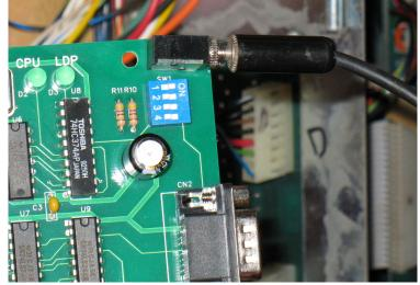
In Direct Wire mode, your LaserCon board needs to connect to +5Volts. The alligator wire must match this photo...
