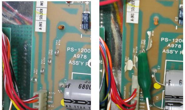
\*\*\*LaserCon has a redundant ground loop through the player cable and audio jacks. Connecting the alligator clip to any test point other than GND will blow fuses.\*
