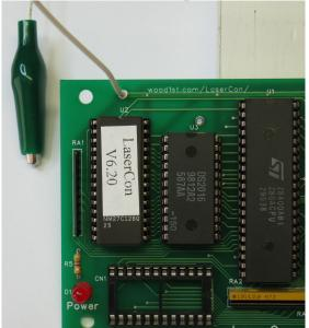
Find the +5Volt test loop on the power supply board.
