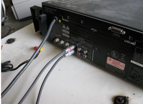
Attach "Audio Out (L and R)" to the GSI board. Attach the 15-pin connector of the LaserCon interface cable to the back of the player.
